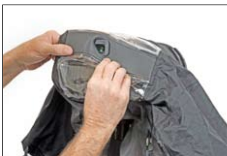
Step 6b: Take the rubberized back off of the eyepiece.
