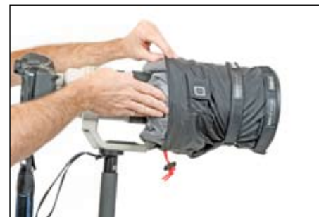
Step 3: Roll up cover underneath the pre-mounting sleeve.
